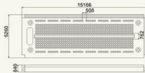
1 Terminal Strip, Tie-point 550 Board: 15*5.3*0.85(cm)
