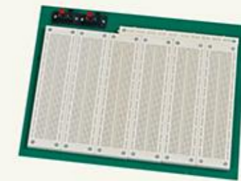
6 Terminal Strips, Tie-point 4560; 1 Distribution Strip, Tie-point 100 Board: 27.7*20.2*0.85(cm) Plate: 30*24*0.3(cm)
